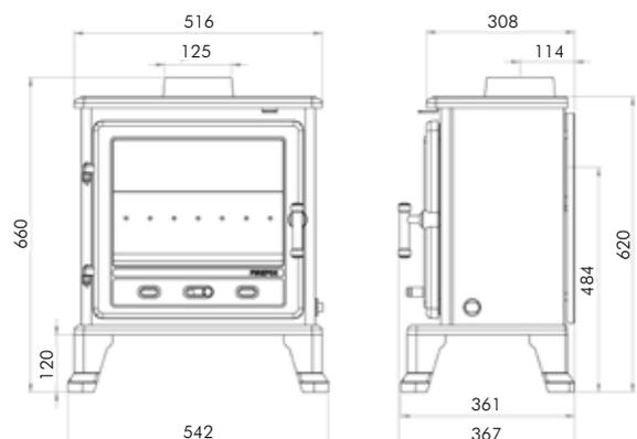
Please see the table on page 91 for installation details in relation to the flue configuration of our stoves, specifically in relation to top and rear flue outlets. The Tiger Gas and Firefox 8 Gas models have a 150mm flue collar but require a 125mm flue. The collar should be packed with rope/fire cement or sleeved with a 6" vitreous pipe to finish.
