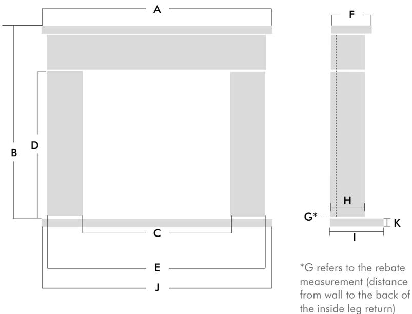
\*G\* refers to the rebate measurement (distance from wall to the back of the inside leg return)
