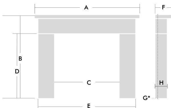
\*G refers to the rebate measurement (distance from wall to the back of the inside leg return)
