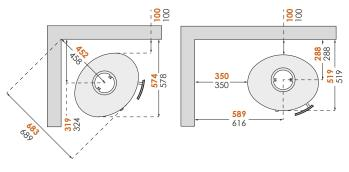
In order to avoid discolouration of painted and treated surfaces, TermaTech recommends the same distance from flammable materials as for non-flammable materials. This distance increases the convection itself around the stove and also eases cleaning. All distances relate solely to the distance of the stove from flammable materials. No account has been taken of national requirements for the use of stove flues or their distance from flammable materials.
